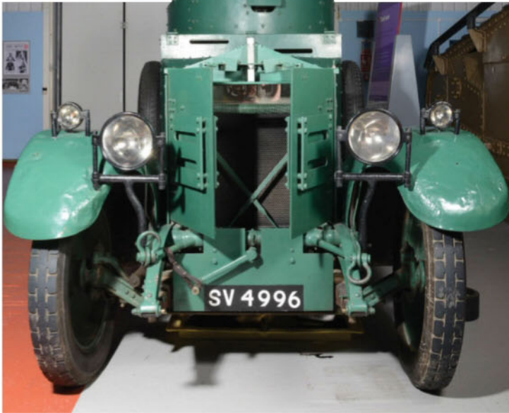
The front of the vehicle could be vulnerable due to the lack of armour on the tyres
